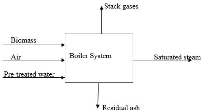
Figure 2. A schematic of the boiler system indicating all material flows
