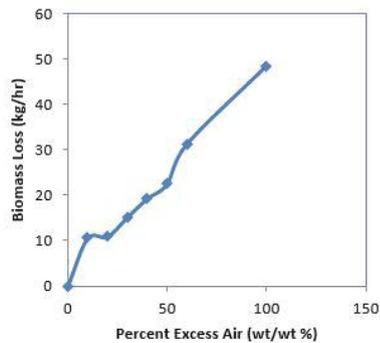
Figure 6. Excess air vrs fuel lost
