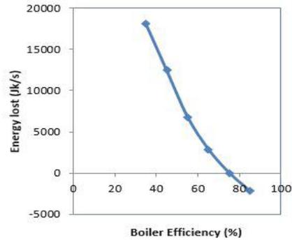
Figure 10. Boiler efficiency vrs energy lost
