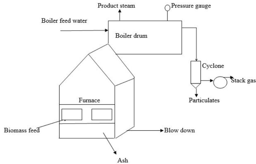
Figure 1. A schematic of the biomass fuelled boiler system [Achaw & Afriyie, 2014]
