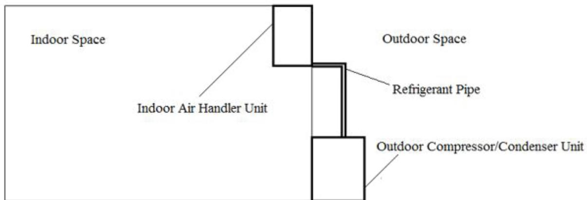
Figure 1: Schematic of a typical Split Unit AC
